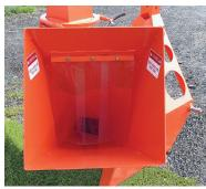
Large 4" x 5" infeed opening, means less pruning and trimming Clear debris curtain strips help protect the user from fly back of material.
